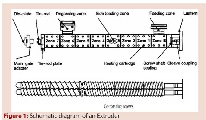
Figure 1: Schematic diagram of an Extruder.
